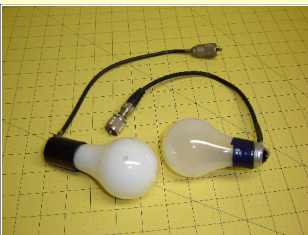
These are two light bulb dummy loads. The left one has a screw-in socket for the bulb. The right one has the coax soldered directly to the bulb center button and the threaded base. While I haven't broken the bulb yet. I put a socket and cable together the make it easier to change bulbs if I did.
