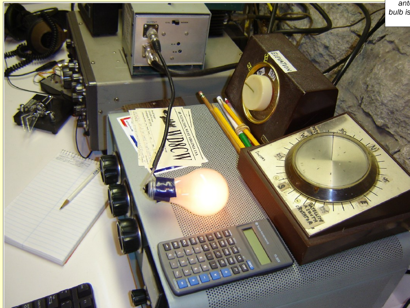
The bulb is not as brightly lit when the Kenwood is in "tune" position. It is easy to see the change in illumination which is a good indicator of RF power.
