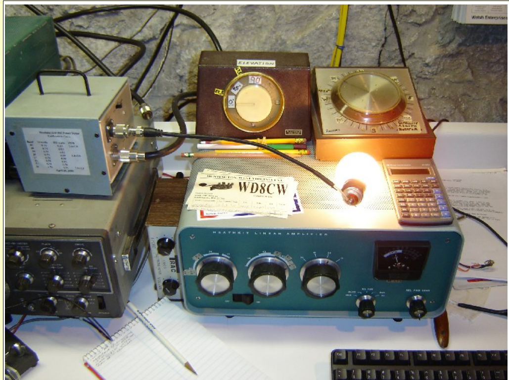
The bulb is connected to the output of a Heath SWR meter. The Kenwood is running about 100 watts and the bulb is very bright. The SWR meter indicated about 1.1 to 1 so the bulb is a good match.
