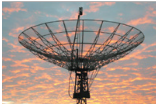
Zdenek Samek, OK1DFC homebrewed this 10 meter dish and feed. Zdenek made the top score on 1.2 GHz with 111 QSOs and 45 multipliers. [Zdenek Samek, OK1DFC, photo]
