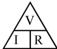
For example if you have a 12 volt battery across a 6 ohm resistor the current flowing would be 2 amperes.
