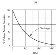
The voltage across the capacitor will rise to 63.2 % of the applied voltage in one time constant. The time constant in seconds is calculated by multiplying the resistance in megohms by the capacitance in microfarads.
