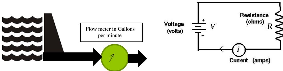
If we know the voltage and the resistance we can calculate the current that would be flowing in amperes using the following expression:
