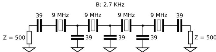
Crystal filter with four crystals ("crystal ladder")
