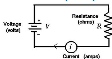
How much power would an electric Iron connected to a 120 RMS AC voltage dissipate if the current flow was 10 amperes?
