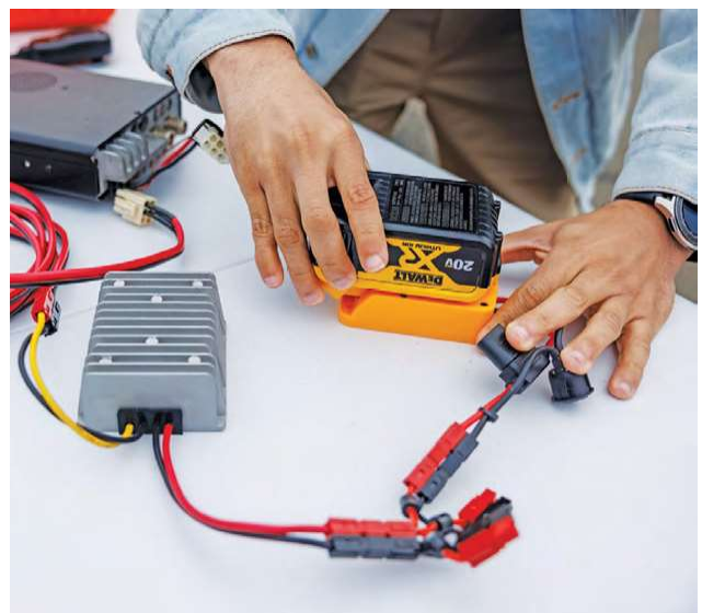
Figure 1 — When setting up for emergency communications, it can be helpful to have battery connectors of multiple brands to maximize your backup power options. A combiner for multiple batteries with Schottky diodes can also be used. [Chris Zajac, photo]
