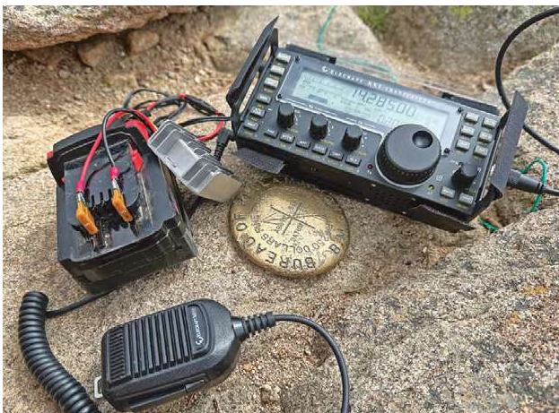
Figure 2 — Gordon S. Novak, Jr., AF5KA, uses ATC fuses to plug into his Milwaukee M18 battery for QRP Summits on the Air operations. A 20 V 8 Ah battery will power a 100 W transceiver for a few hours [Gordon S. Novak, Jr., AF5KA, photo]
