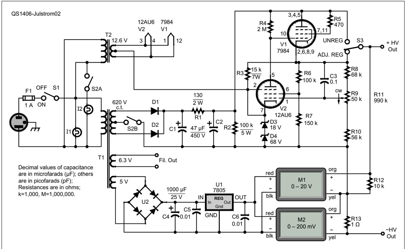
Figure 2 — Circuit of the HV supply with a tube-based adjustable regulator.
