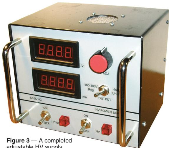
Figure 3 — A completed adjustable HV supply.
