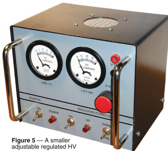
Figure 5 — A smaller adjustable regulated HV supply with analog meters.
