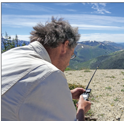
Figure 4 — Rob, AE7AP, uses the VX-8DR with a Pryme AL-800 telescopic antenna to send an APRS message from the Continental Divide.
