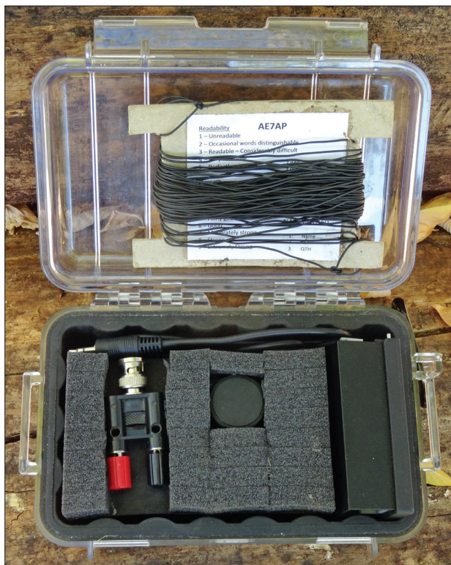
Figure 2 — The KX1 in its Pelican 1050 case with the PPK straight key, earbuds, and antenna.
