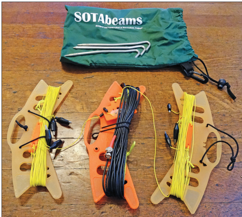
Figure 8 — The SotaBeams 20-30-40 link dipole kit.
