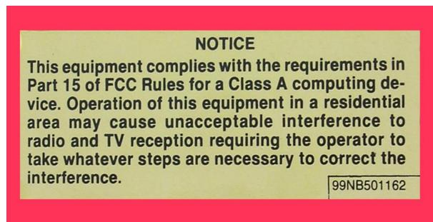
Figure 20 Radio-Interference Label from a Class A Device
