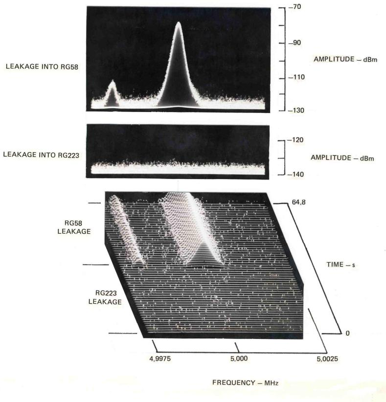
Figure 10    Example of Leakage into Coaxial Cables
