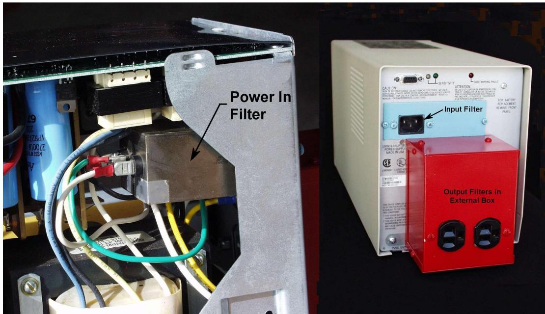
**Figure 46    UPS Modified to Comply with BFG Principles**
