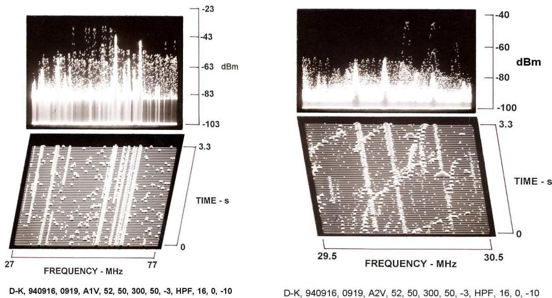
**Figure 32 Intermittent Interference from Frequency-Hopping and ISM Emissions**
