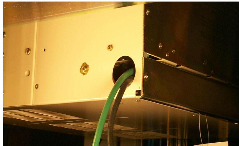
**Figure 50    Unfiltered Conductors Exiting a Switching Power Supply**
