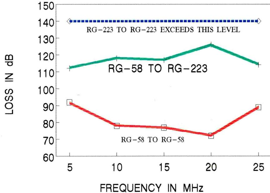
**Figure 11**    **Cable-to-Cable Coupling Loss**
