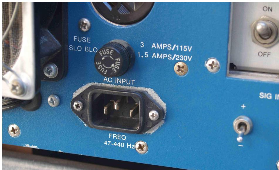
**Figure 47** Power Connector that Complies with BFG Principles
