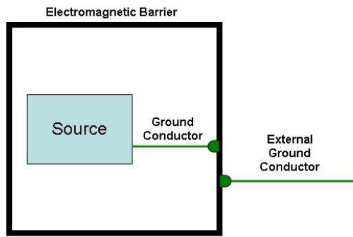
**Figure 40     Barrier Treatment of a Ground Conductor**
